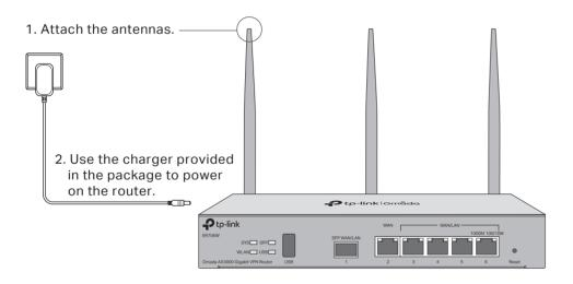
4. Wait until the SYS LED flashes slowly and the WLAN LED turns solid, indicating the router is ready for setup.
